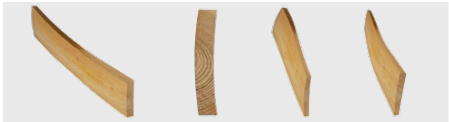
Blocks with longitudinal/latitudinal deformation, cupped or warped
