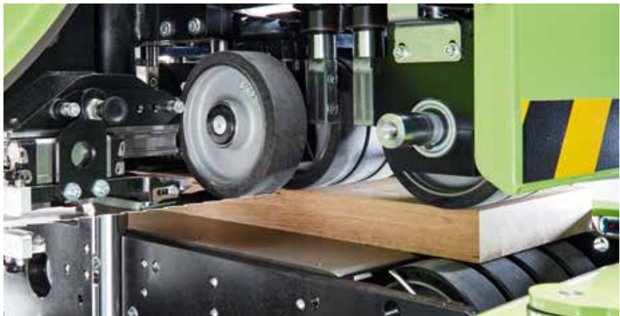
Driven feed rollers at top and bottom
